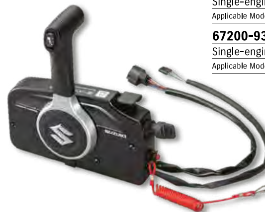
67200-91J20-000 Single-engine Applicable Model DF4-6
